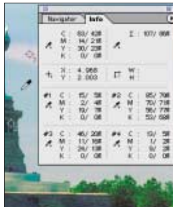
Figure 2.6 When a curve or other adjustment dialog is open, the Info palette shows before-and-after values, separated by a slash. Users also can define, using the color sampler tool, up to four fixed sample points, which will update continuously as the correction proceeds.
